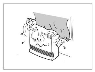
Flue fittings must be kept clear of flammable materials.
